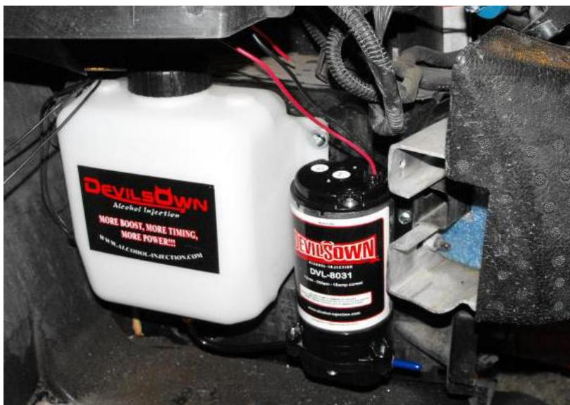
Figure 2: Pump placement
