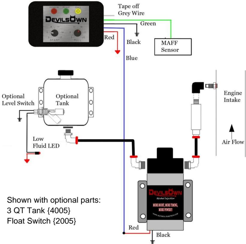
Figure 4: Kit Wiring Diagram
