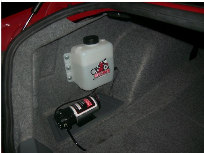
Figure 2: Pump placement
