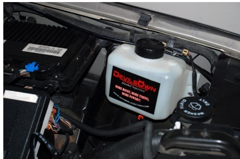
Figure 1: Tank Placement
